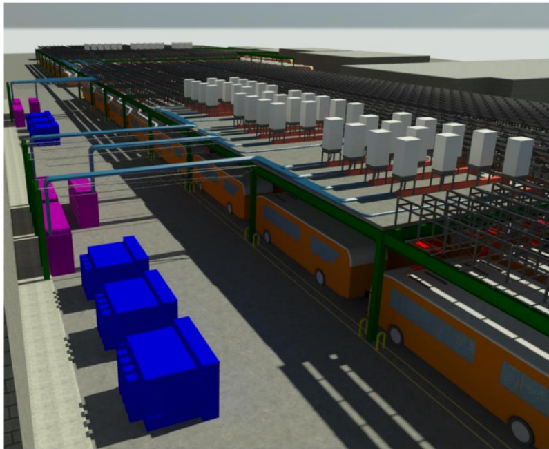
Figure 6: Design Rendering of Charging Infrastructure Layout for LA Metro
